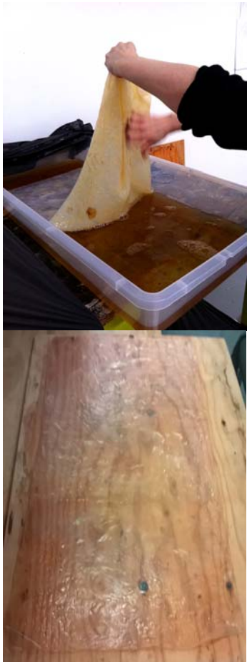
Figure 4: Removing and drying the living tissues after a 3 week growth period in a static culture.
